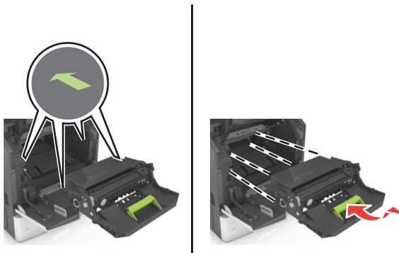
**Note:** Use the arrows on the side of the printer as a guide.
