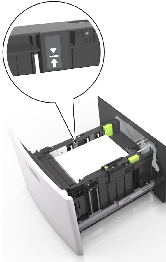
**Warning—Potential Damage:** Overfilling the tray can cause paper jams.
