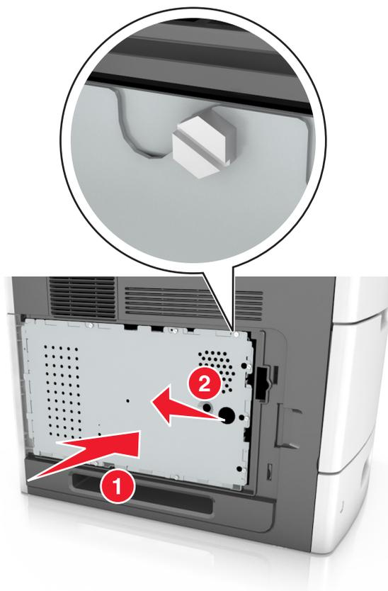
6 Tighten the screws on the shield.
