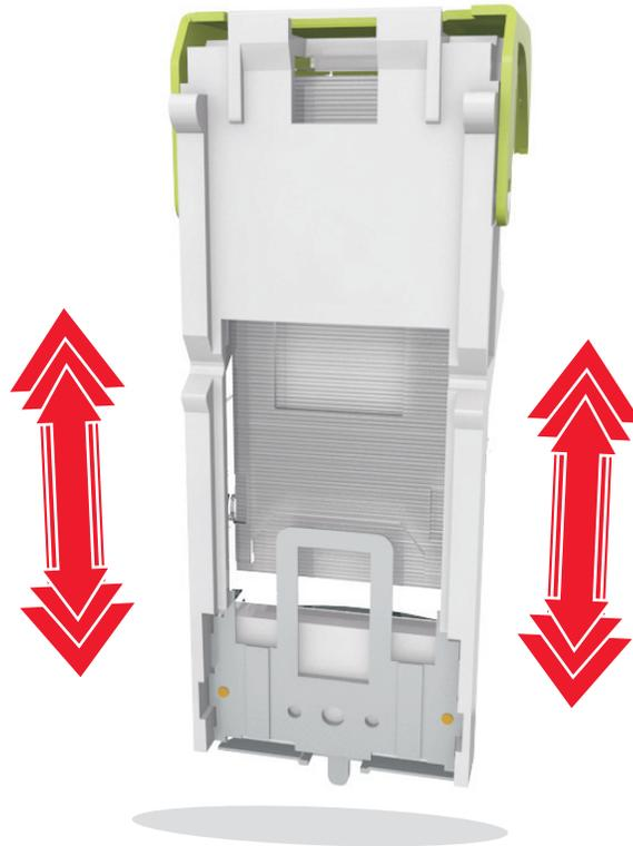
**7** Push the cartridge holder firmly back into the stapler unit until the cartridge holder *clicks* into place.
