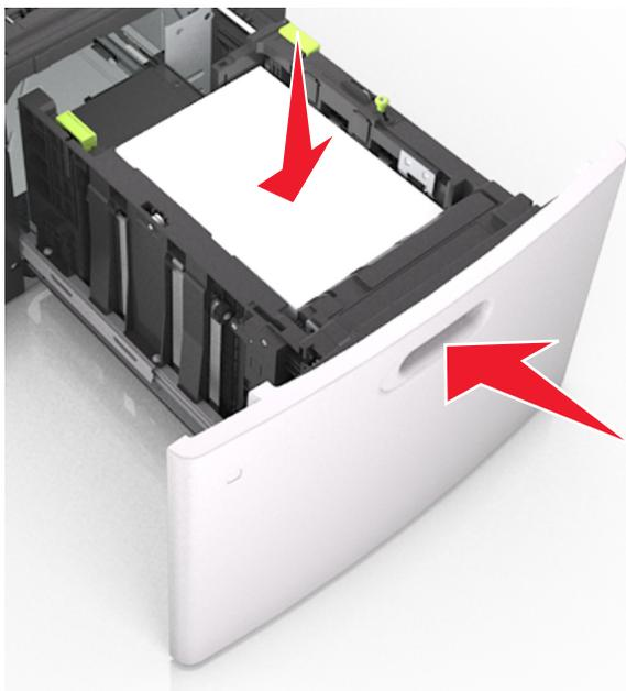
**6** From the printer control panel, set the size and type in the Paper menu to match the paper loaded in the tray.
